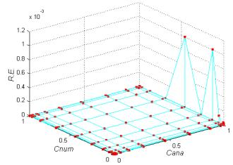
Fig. 8: Behaviour of relative Error for Pe=60 with 15 elements
