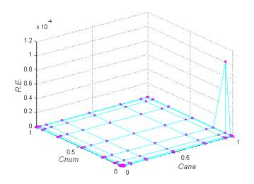
Fig.10: Behaviour of relative Error for Pe=100 with 50 elements
